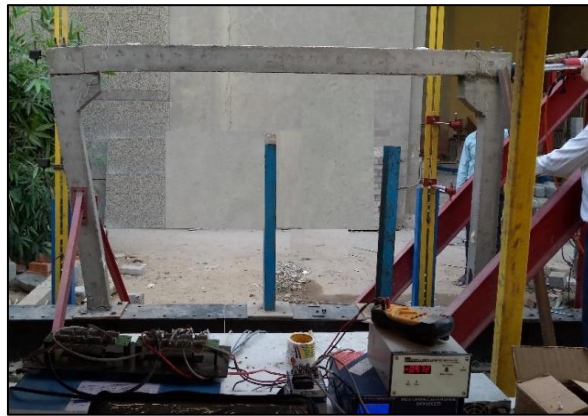
Figure 18. Failed specimens with maximum lateral displacement
